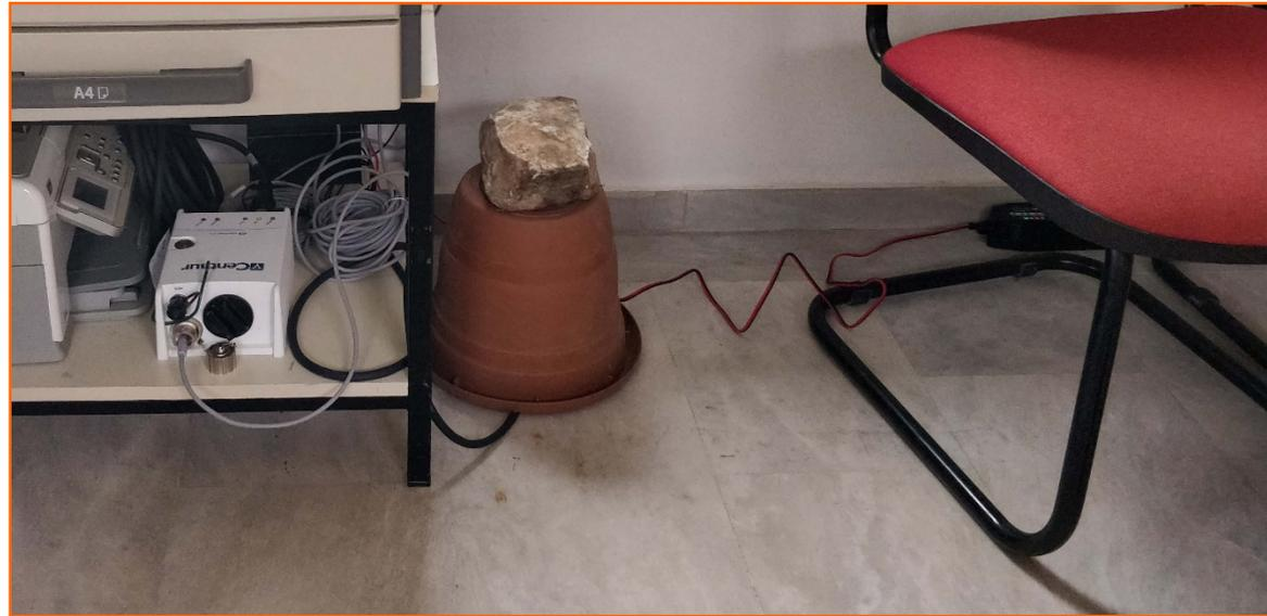
Indicative images from the installed seismographs of the temporary network for monitoring the post-earthquake sequence of the Tyrnavos – Ellassona earthquake.
