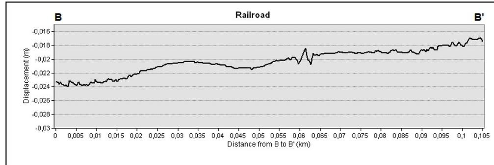
Histogram showing the deformation along National Railway Network. An anomaly was observed due to noise signature.
