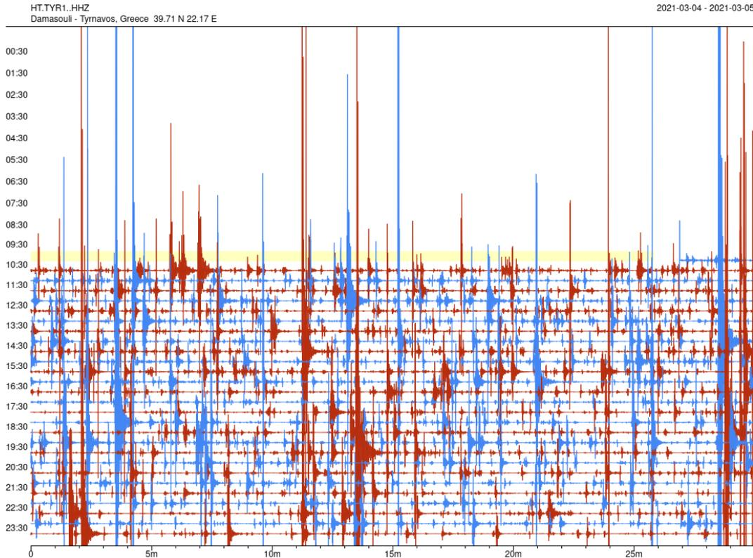
Drum plot of the temporary seismological station TYR1 of the seismic network for monitoring the aftershock sequence of Tyrnavos - Elassona
